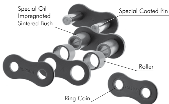
Fig. 22 Basic Construction
