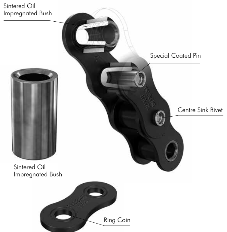
Fig. 10 Basic Construction
